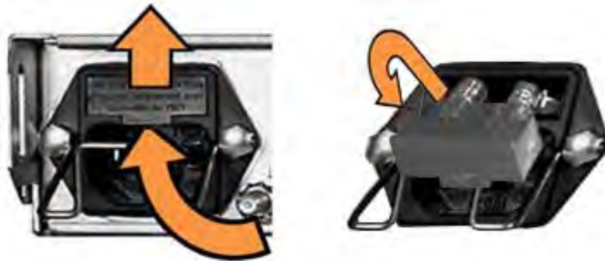
Figure 4-6. Replace the AC Fuses
