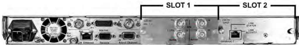
Figure 1-2. CDM-710/L Rear Panel Data Interface Slots
