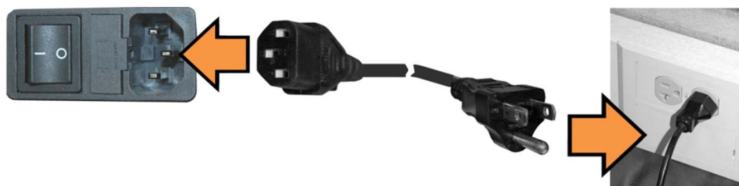
Figure 3-8. Applying AC Power to the CDM-750
