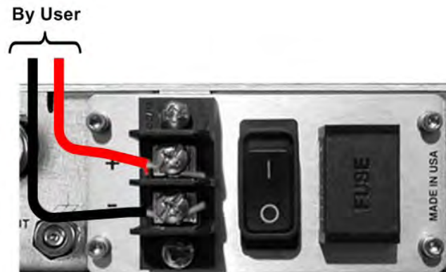
Figure 3-10. Apply DC Power to the MBT-5000
