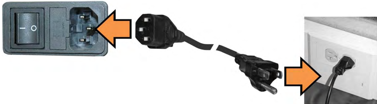
Figure 3-6. Apply AC Power to the MBT-5000
