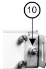
Figure 4-12. Unit Ground Connection
