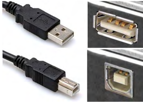
(TOP) Type 'A' USB Plug and Receptacle (BOTTOM) Type 'B' USB Plug and Receptacle
