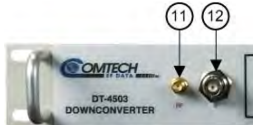
Figure 4-14. Front Panel Sample Test Point Connections
