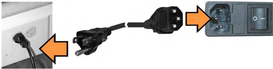
Figure 4-9. Apply AC Power to the Unit
