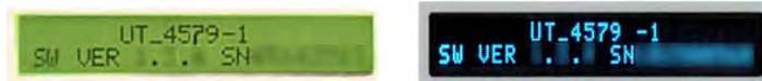
(LEFT) Liquid Crystal Display (LCD) – Initially Released Chassis (RIGHT) Vacuum Fluorescent Display (VFD) – Current Production Unit
