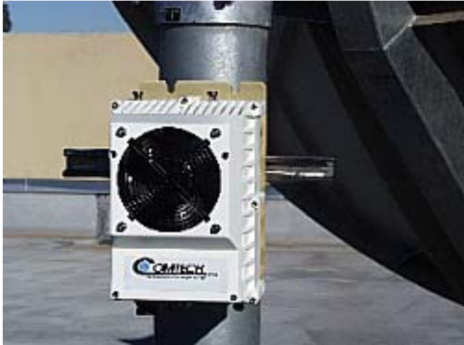
Figure A-7. Mounting XSAT Unit
